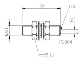
Inductive Sensors BES 516-378-E4-C-PU M8x1 x 30 normally-closed Sn=1,5mm shielded
